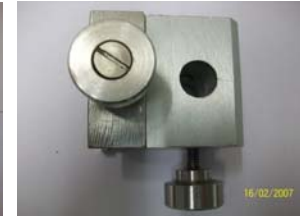
Rail slider(13mm dia bore)
